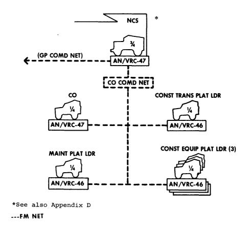
Figure 12-5. Type radio net, engineer light equipment company, airborne.
