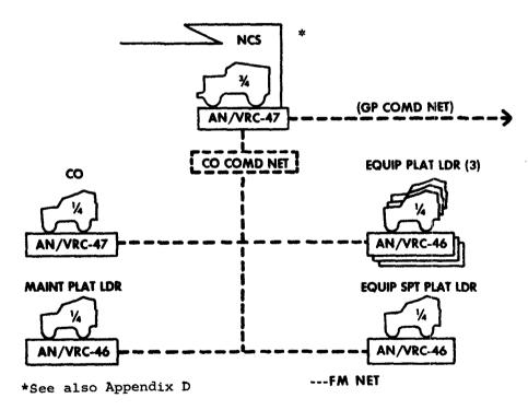
Figure 12-2. Type radio net, engineer light equipment company.
