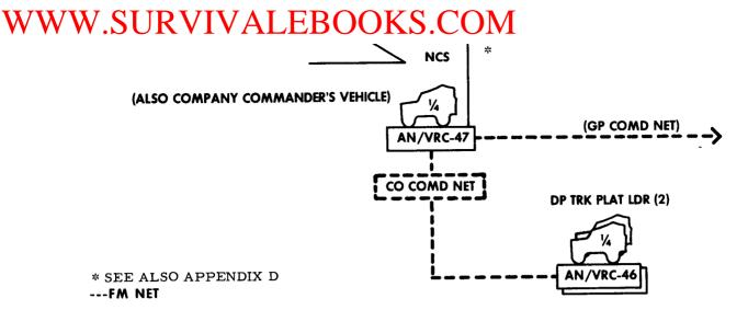
Figure 13-2. Type radio net, engineer dump truck company.
