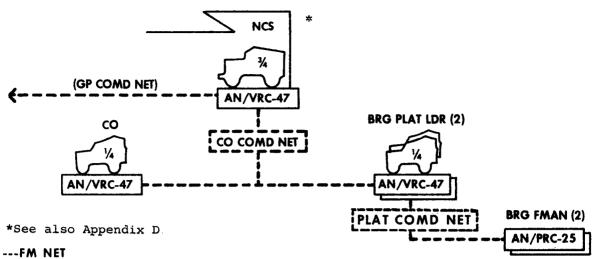
Figure 11-2. Type radio net, engineer panel bridge company.
