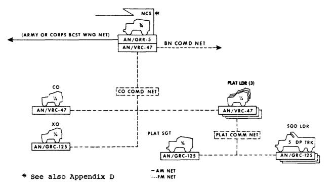
Figure 8-6. Type radio net, engineer combat company, engineer combat battalion, army or corps.
