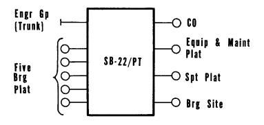
Figure 10-3. Type wire net, engineer float bridge company.
